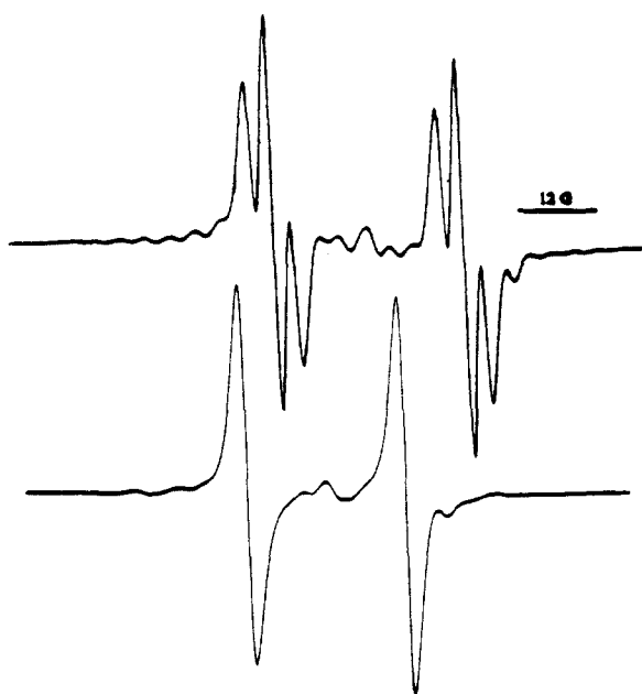
Figure 4. EPR spectra at 250 K of (upper) 6 and of (lower) the PhSiD 2 analogue, in toluene. Gain, 6; modulation intensity, 0.2 G.
